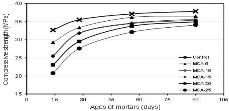
Figure 09: Compressive strength at different ages of mortars containing some ash B
