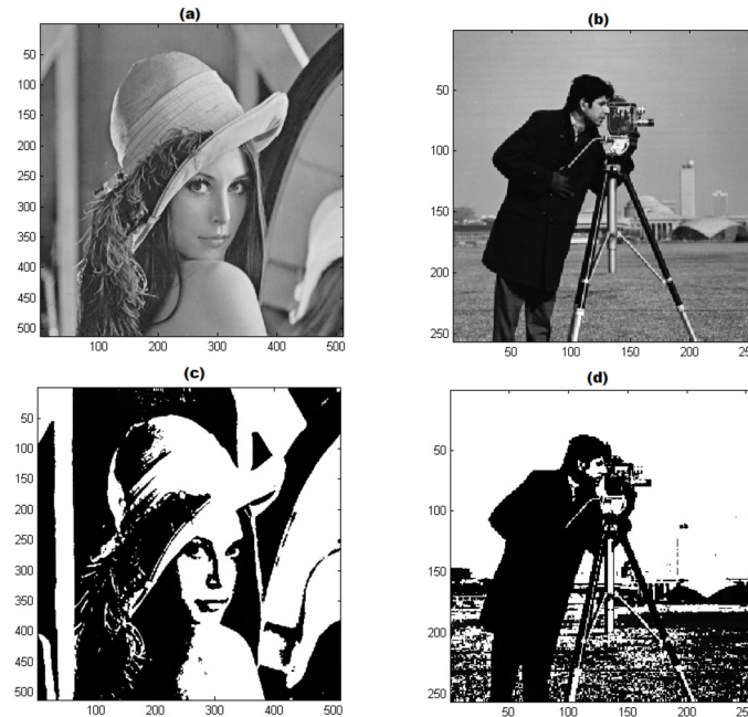
Figure 12. (a) and (b) are the original images; (c) and (d) are their images segmented by the generalized nonlinear anisotropic diffusion model, with the values of the parameters of the model: a = 10 ; n = 3 ; \rho = 1.5 ; t = 2 ; dt = 0.01 ; k = 0.03783 .
