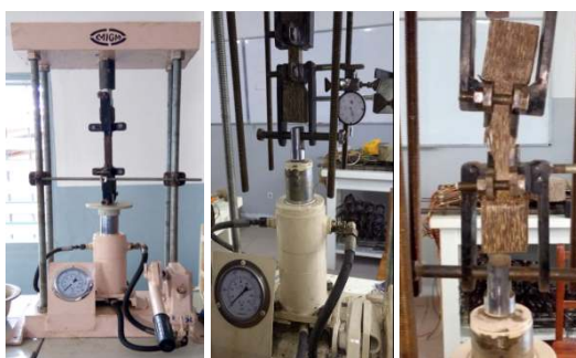
Fig. 4. Placement of the test specimen; beginning and end of the direct tensile test
