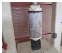
Fig. 2. Start of compression test on hydraulic press
