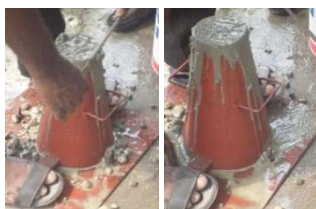
Fig. 1. Subsidence test in progress
