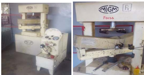
Fig. 3. Beginning and end of the four-point bending test
