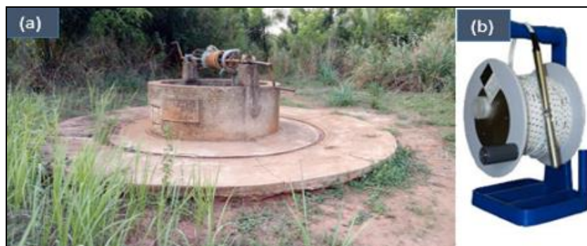
Figure 3. Figure showing field equipment: (a) modern well at Ayomi in Dogbo township; (b) piezometric probe
