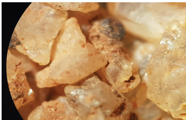
Figure 12: Optical microscope observation of the bar earth of Abomey-Calavi
