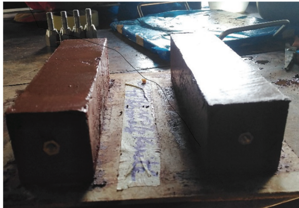
Figure 6: 4 \times 4 \times 16 specimens with inserted studs
