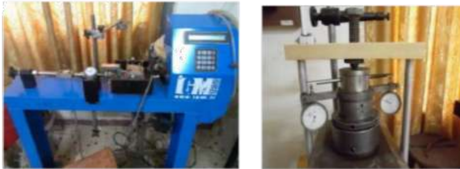
Figure 2:- Shear apparatus equipment and oedometer cell for humidification.
