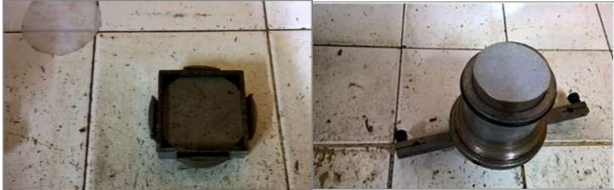
Photo 1:- Extraction of the sample from the oedometer cell Photo 2:- Coring the wetted sample.
