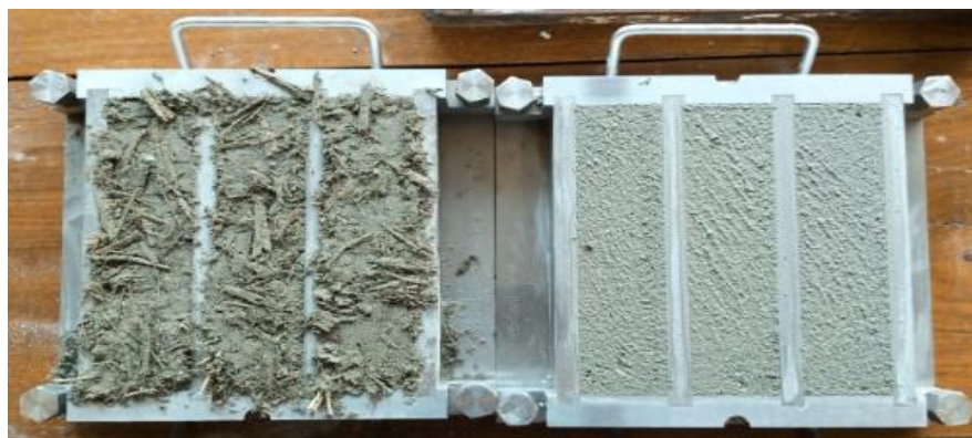
Figure 9 : Molding of test pieces
