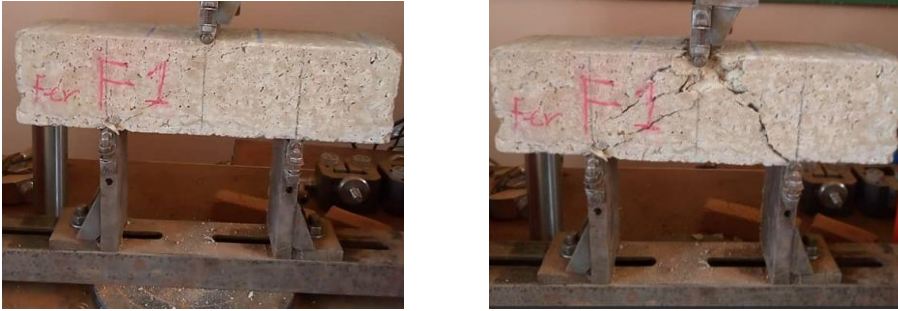
Photo 5:- Beam 10cm x 10cm x 40cm in unreinforced reinforced concrete (witness beam).
