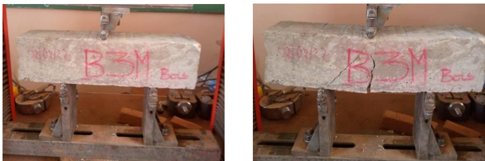
Photo 4:Beam 10cm x 10cm x 40cm in concrete reinforced with oppositifolius mallotus wood.
