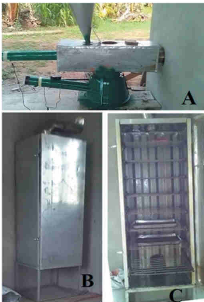
Figure 1. Smokehouse ATINGAN® A: Heat generator, B: Closed smoking chamber, C: Open smoking chamber.
