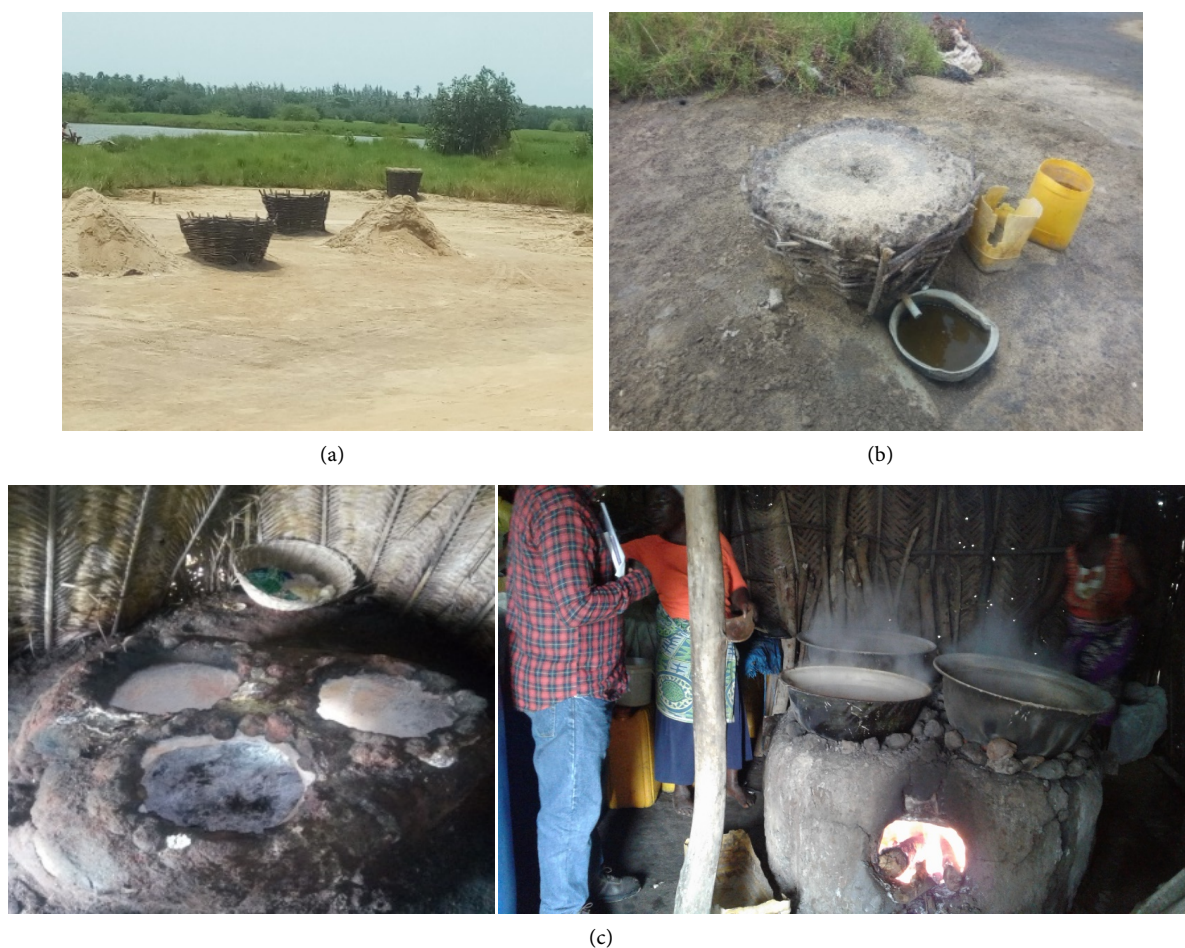
Figure 3. Photo 2: (a) Salty sand collecting field at Djègbadji; (b) Extraction of salt water by leaching salty sand; (c) Preparation of salt at Djègbadji (Ouidah)/usage of three-burner ovens.
