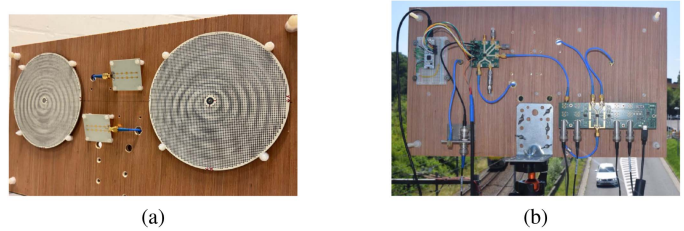
Fig. 4. Illustration of the FMCW radar system. (a) Front view: antennas part. (b) Back view: system part. The top left green board is the transmitter (BGT24MTR11 from Infineon [25]) connected either to the Tx serial patch antenna or to the Tx MTS antenna. A copy of the Tx signal is used as the local oscillator for the dual receiver (BGT24MR2 from Infineon [26]) and its associated baseband amplifiers and filters on the bottom right board. The Rx serial patch antenna and the Rx MTS antenna are both connected to the dual receiver to ease the comparison. The generation of the calibrated signal used to tune the integrated oscillator for the frequency modulation, and the data acquisition are performed by a PicoScope 3404D from Pico Technology [27].
