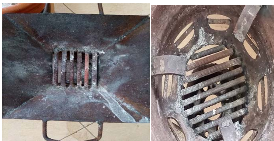
Figure 15. Square door (left) and rimmed stove (right) after durability test.
