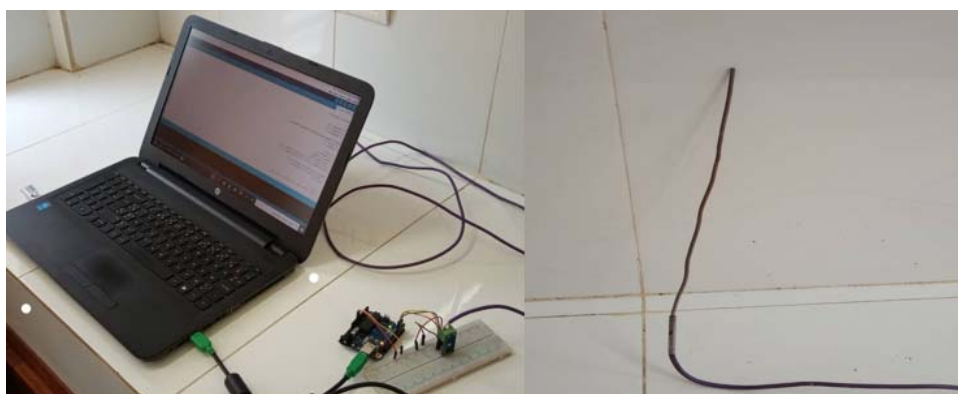
Figure 6. Data acquisition system + thermocouple.
