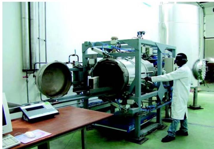
Figure 1 – experimental apparatus for thermal treatment and D.D.S drying devised plant for the waterlogged woods treatment for conservation.
