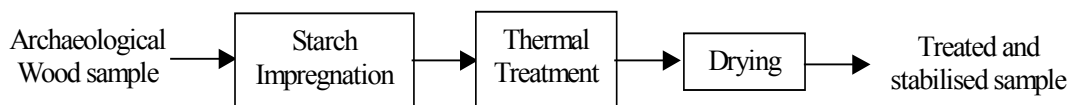
Figure 1. Sequences of the process developed by Sanya et al., (2000) for the conservation of waterlogged woods
