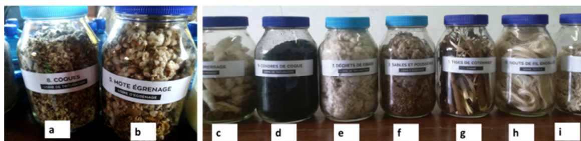
Figure 10. Photo of by-product samples: (a) hulls, (b) ginning clods, (c) destoning's clods, (d) hulls ashes, (e) fiber waste, (f) sand and dust, (g) cotton stalks, (h) glued thread's bits, (i) thread's bits.
