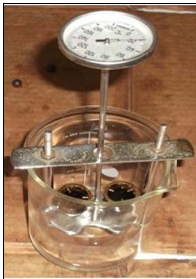
Figure 3. Ring and Ball standardized testing device used for softening point measurements.
