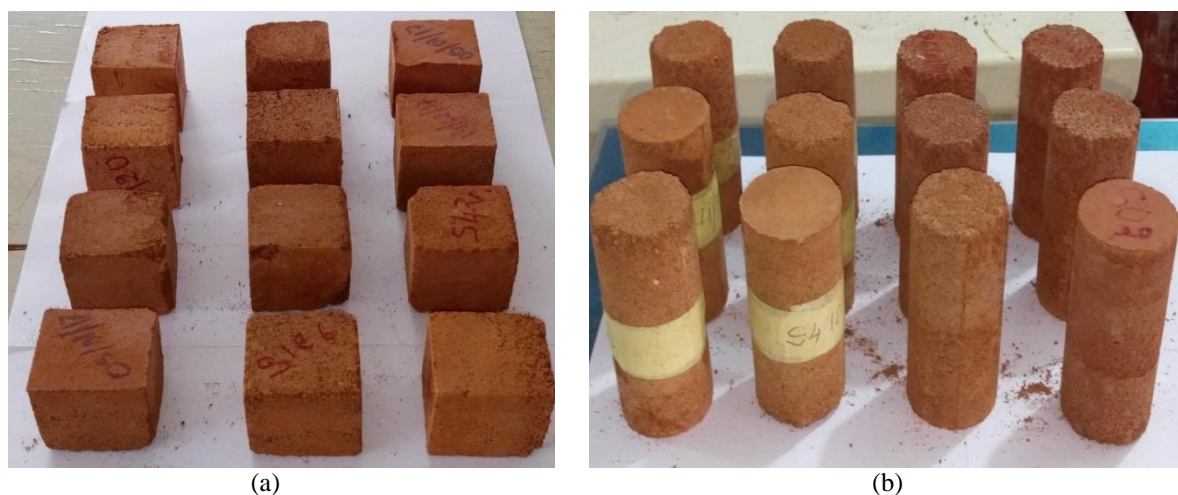
Figure 3 – Test tubes made for the tests of compressive strength: (a) - cubic, (b) - cylindric
