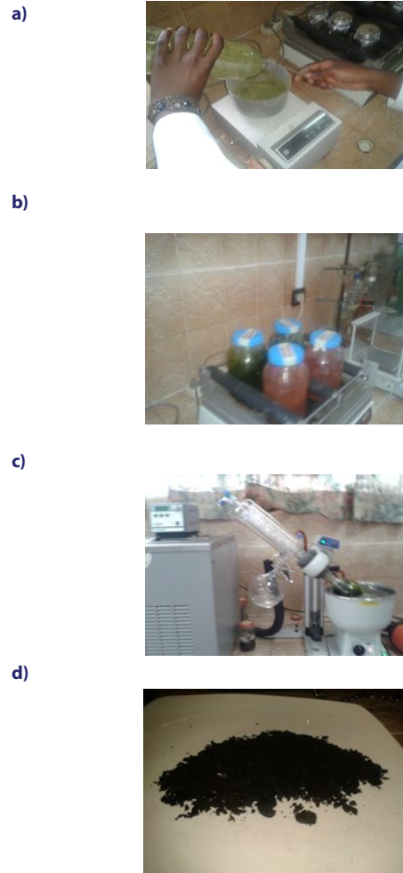
Figure 7. Extraction Process on leaves of Annona muricata (a: Weight of the powder of the leaves; b: powder mixed in ethanol 90 ° with stirring; c: filtrate mixture leaf powder / ethanol 90 ° evaporation the ROTA VAPOR d: extracts from the leaves of Annona muricata dried and crushed) (Photo Natacha AIVODJI 2014).
