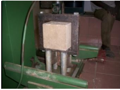
Figure 6: Conduct of the direct tensile test
