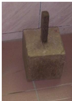
Figure 4: Concrete cube specimen of 16cm lateritic nodules of ridge and reinforced in the central part
