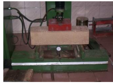
Figure 5: Execution of the 4-point bending test
