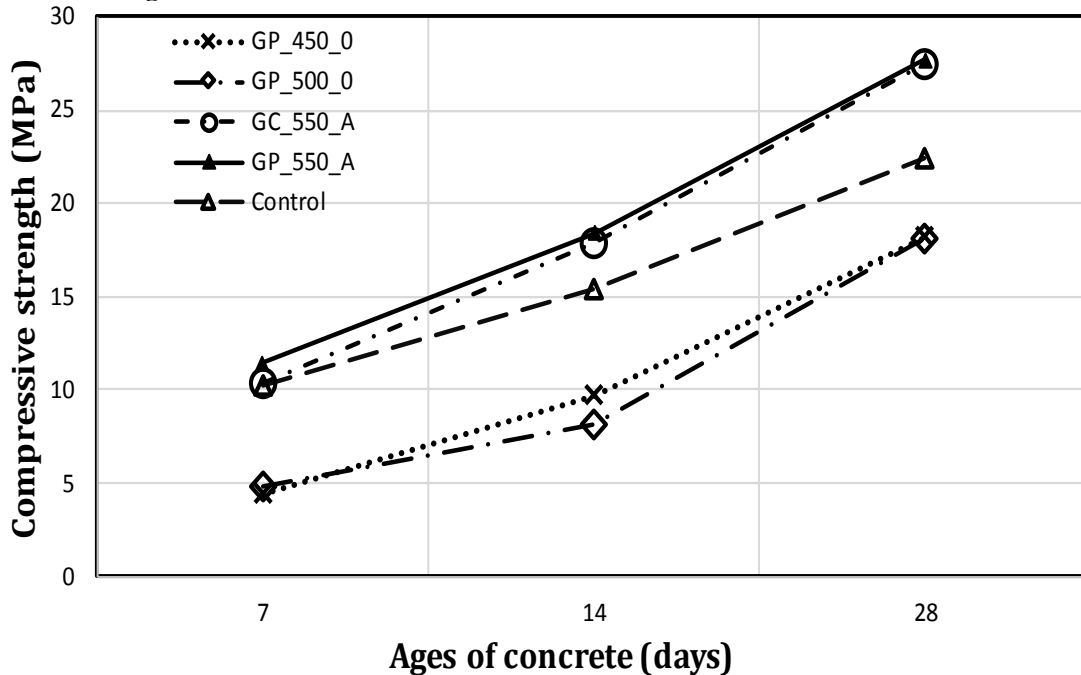
Figure 06:- Variation in compressive strengths of different types of concrete over time.
