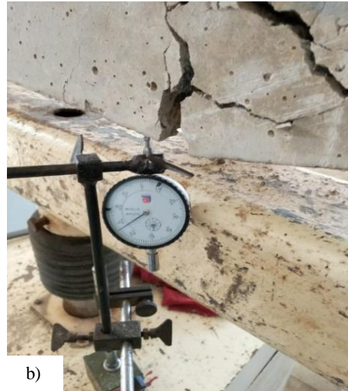
Figure 05:- Appearance of the beams in the 4-point bending test : a) Beam placed on the press before testing b) Condition of the beam after testing and reading the deflection.
