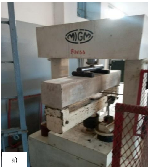
Figure 05:- Appearance of the beams in the 4-point bending test : a) Beam placed on the press before testing b) Condition of the beam after testing and reading the deflection.
