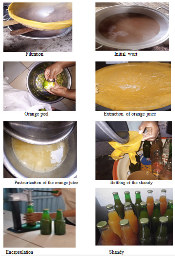
Figure 3) Images showing the filtration of the brew to obtain the initial wort, certain operations for the orange juice extraction and operations for conditioning and stabilizing the shandy
