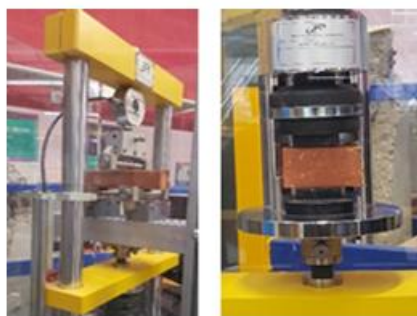
three-point bending tests
