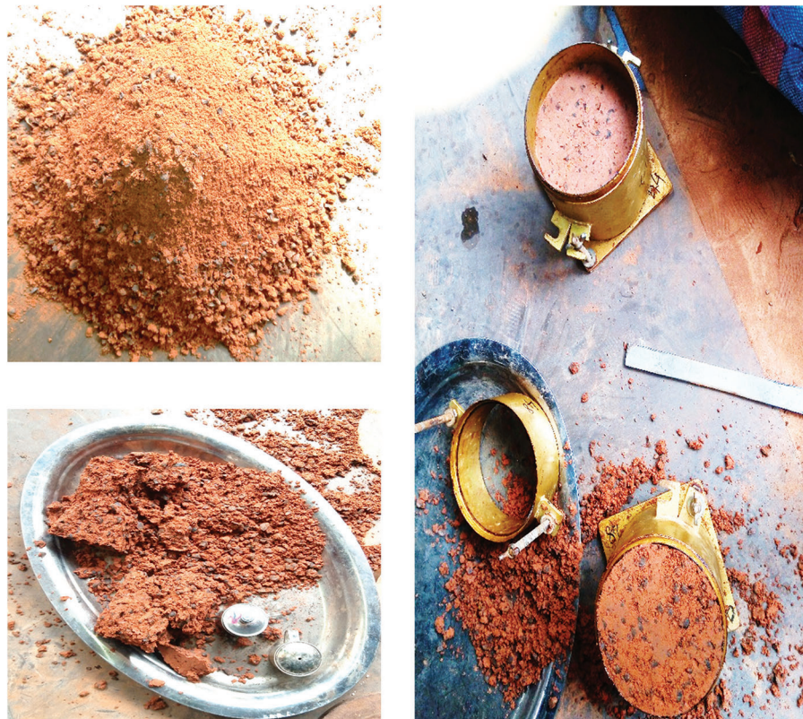
Figure 3: Study images of mixtures (lateritic soil + PKS)
