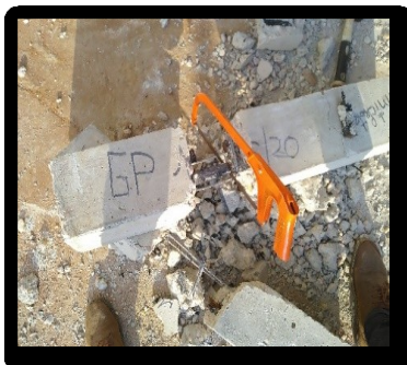
Figure 14 :- Extraction of the treated Borassus frames
