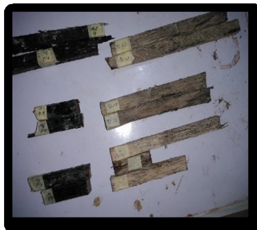
Figure 15:- Sample of Borassus wood extracted from concrete for steaming
