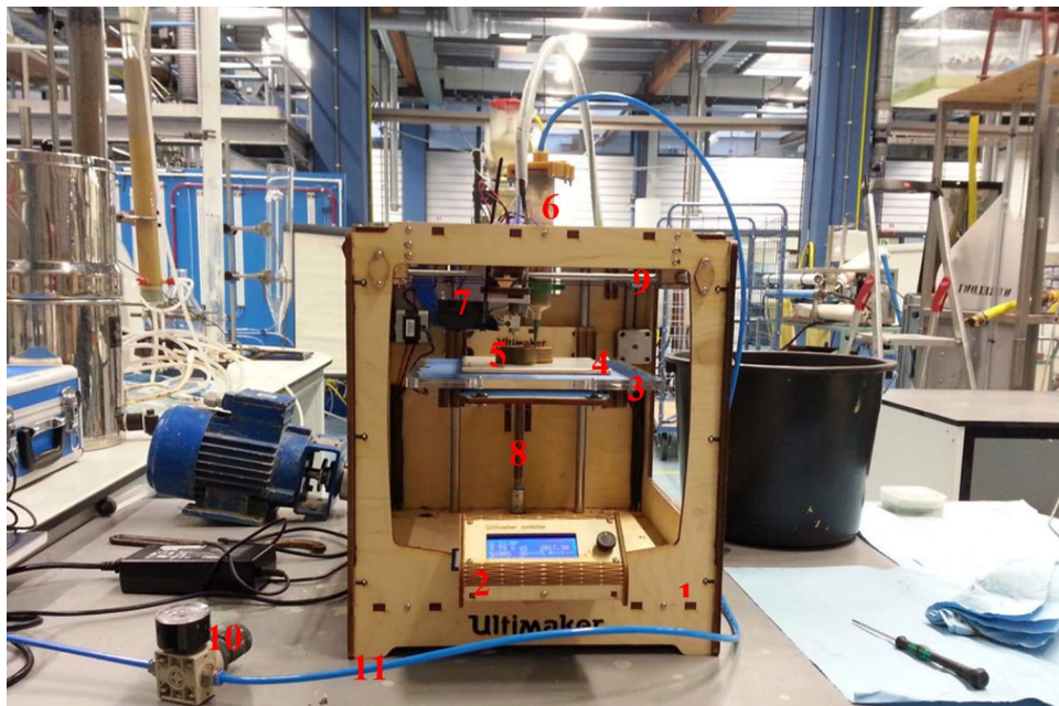
Fig. 3 Overview of the additive manufacturing device dedicated to the realization of the filters. 1. 3D printer “Ultimaker 1”. 2. Device for controlling the printing speed. 3. Printing platform. 4. Ceramic support. 5. In-process materials. 6. Syringe containing ceramic paste. 7. Fan for drying. 8. Actuator. 9. Travel bar allowing movement of the print head. 10. Manometer for pressure control. 11. Pressurized air duct connection
