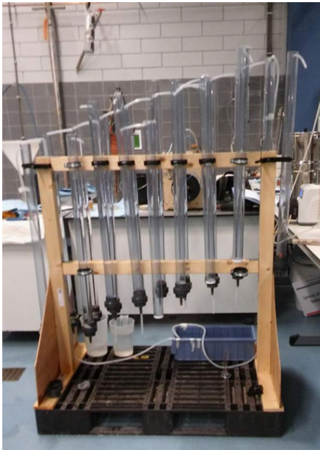
Fig. 4 Experimental setup for water filtration tests
