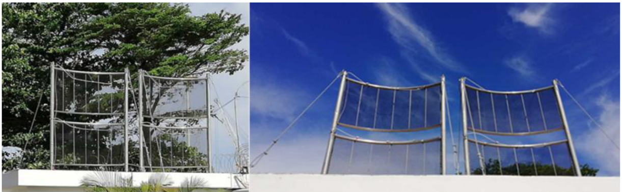
Fig. 4. Four separator units have been constructed and two stacks of 2 m height and 2 m width (each one consisting of two units) have been installed nearby the monitoring equipment on the roof a building located from the German Embassy in Cotonou.
