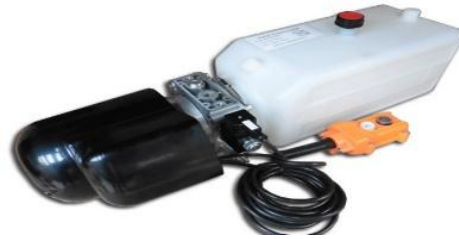
Fig. 14. Mini-hydraulic unit with control box [12]
