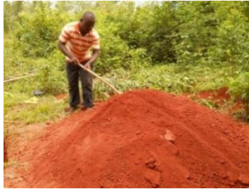
Figure 2:- Quartering on a 1 m pass
