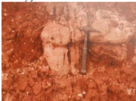
(a) Relics of healthy rock inside alteration materials (b) Clayey soil within sound rock Figure 11 : Healthy rock mix and alteration materials on the Abomey plateau (IRB, 1985)
