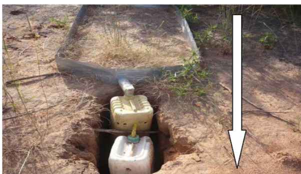
Figure 2. Experimental plots delimited by sheet metal (Erosion plots measurement design).
