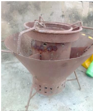
Figure 10. Improved rice husk metal hearth (Kpossilandé, 2022)
