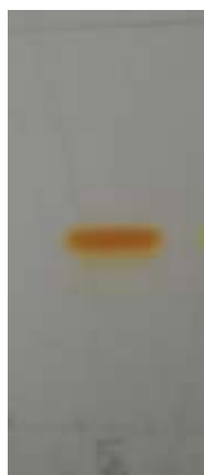
Figure 7:- TLC plate showing furosemide after mobile phase development.
