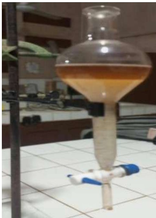
Figure 5:- Separating funnel showing dichloromethane and aqueous fractions.
